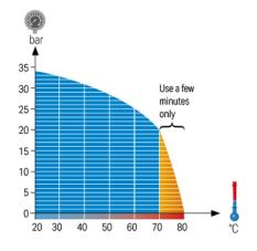
Maximum working pressure 20 bar at 70°C
